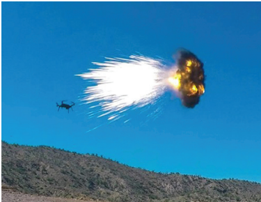
CUAS engagement using Proximity Sensing Ammunition
